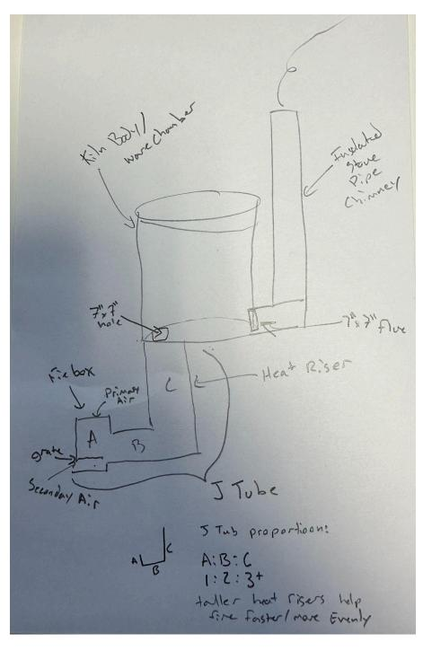
This diagram shows the rough layout and proportions of the parts of the rocket kiln. The proportions of the J tube, heat riser and flue openings are important for the efficient firing of a rocket kiln. This is designed to fire in neutral/oxidation.
